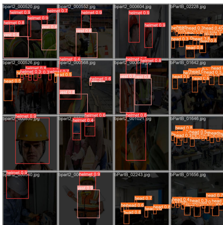
Figure 2: Results of Safety Helmet Detection for Construction Workers at Night
